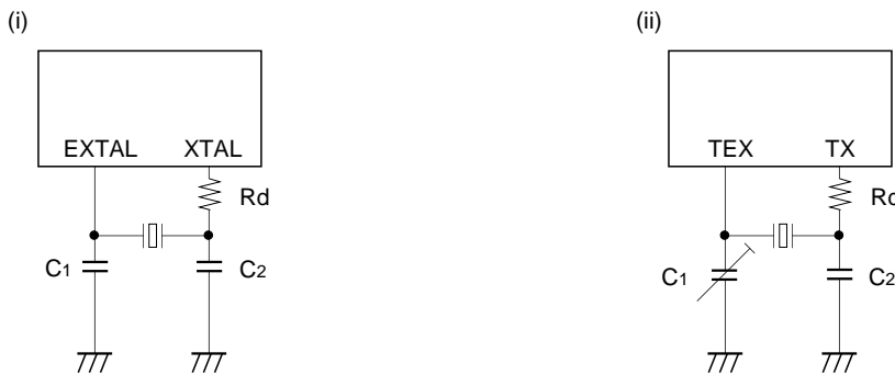
Fig. 13. Recommended oscillation circuit
